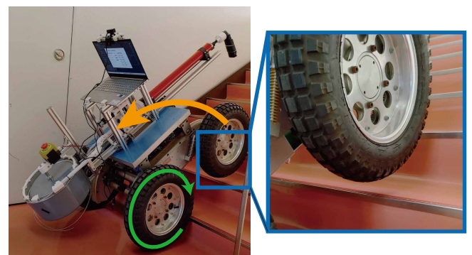
Fig. 7: Experiment of climbing stairs without using ETA. The front wheels were lifted off the ground due to the torque from the spinning rear wheels.
