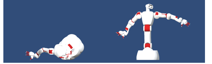
Fig. 4. The physics-enabled robot (left) falls due to real-world constraints, unlike the robot rig (right).
