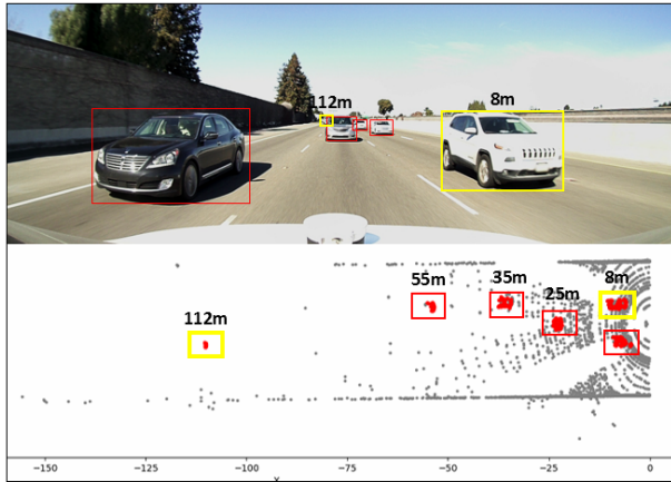
Fig. 5. Qualitative result of proposed method Vehicles were detected from 8m to 112m.
