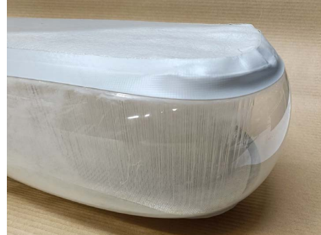
Fig. 1: Transparent balloon sample with an internal drop-stitch structure. The top and bottom surfaces are connected by threads or space yarn to help maintain the shape of the balloon under external forces. Bending, tilting, or deforming is reduced due to force distribution by the threads.
