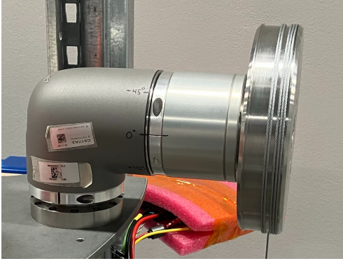
Fig. 6. Test setup with a standalone UR joint with a force/torque sensor and a pulley system mounted on the output flange.
