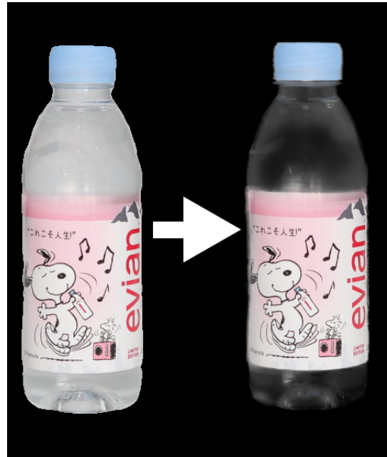
Fig. 1: Processing images for Neural Scanning with a black background applied to the images. Left: Binary segmentation, the background color of the scanning environment becomes part of the object. Right: Result of our transparency estimation pipeline, transparent parts are alpha blended with the image background.
