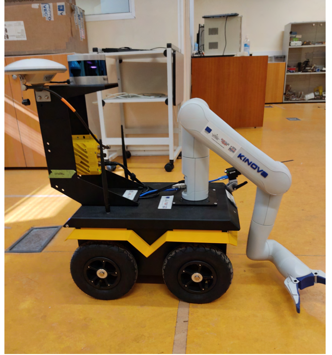
Fig. 4: Jackal with Gen3 lite - The mobile manipulator used for data gathering.
