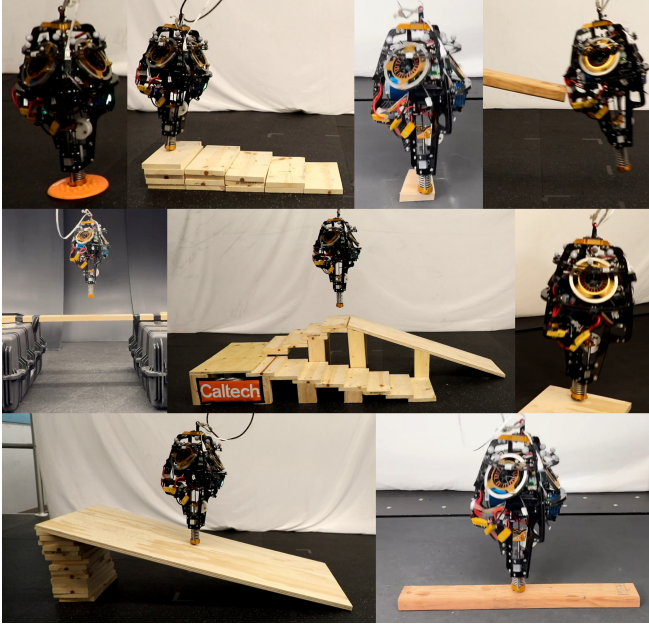
Fig. 4: A snapshot of the experiments conducted with ARCHER, including set point tracking, disturbance rejection, and hopping over rough terrain.
