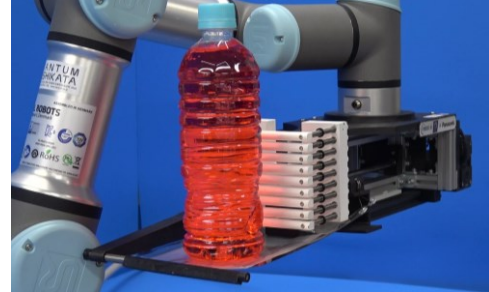
Figure 2. Prototype shown scooping and carrying a 500-mL PET bottle filled with water
