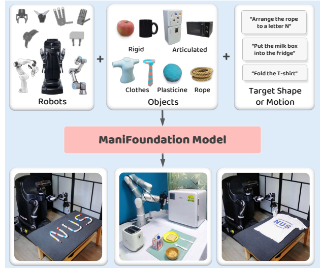
Fig. 1. We propose a ManiFoundation Model that can generalize over a diverse range of robots and objects, and perform various kinds of manipulation tasks based on 3D point cloud input.
