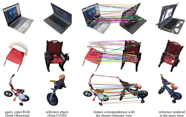
Fig. 4. Qualitative results of Zero123-6D on the Objectron dataset [53]. From left to right: the query RGB image, a reference example, the closest reference view with matched feature points, and finally, the lifted RGB point cloud of the reference in the estimated 6D pose of the query (only for visualization). The reference objects are from CO3D [51].
