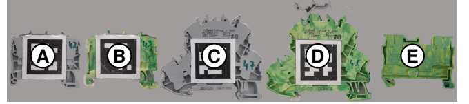
Fig. 4: Tested clamps. The clamps B and D feature a metal foot (higher assembly force), E, C and A a plastic foot.
