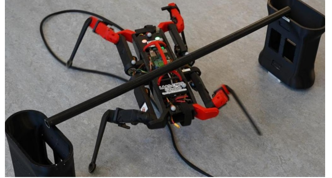
Fig. 5: CaT trained with a constraint that limits the height of the base learns crouching locomotion skills.
