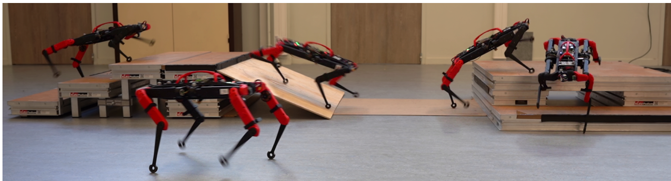
Fig. 1: The open-hardware quadruped robot Solo-12 trained with CaT performing agile locomotion over challenging terrains while satisfying safety and style constraints. The robot can walk up stairs, traverse slopes, and climb over high obstacles.
