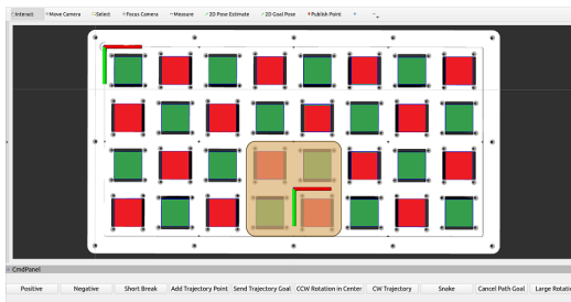
Fig. 7. Interactive 3D model of the 1 \times 2 VERA represented in RViz.
