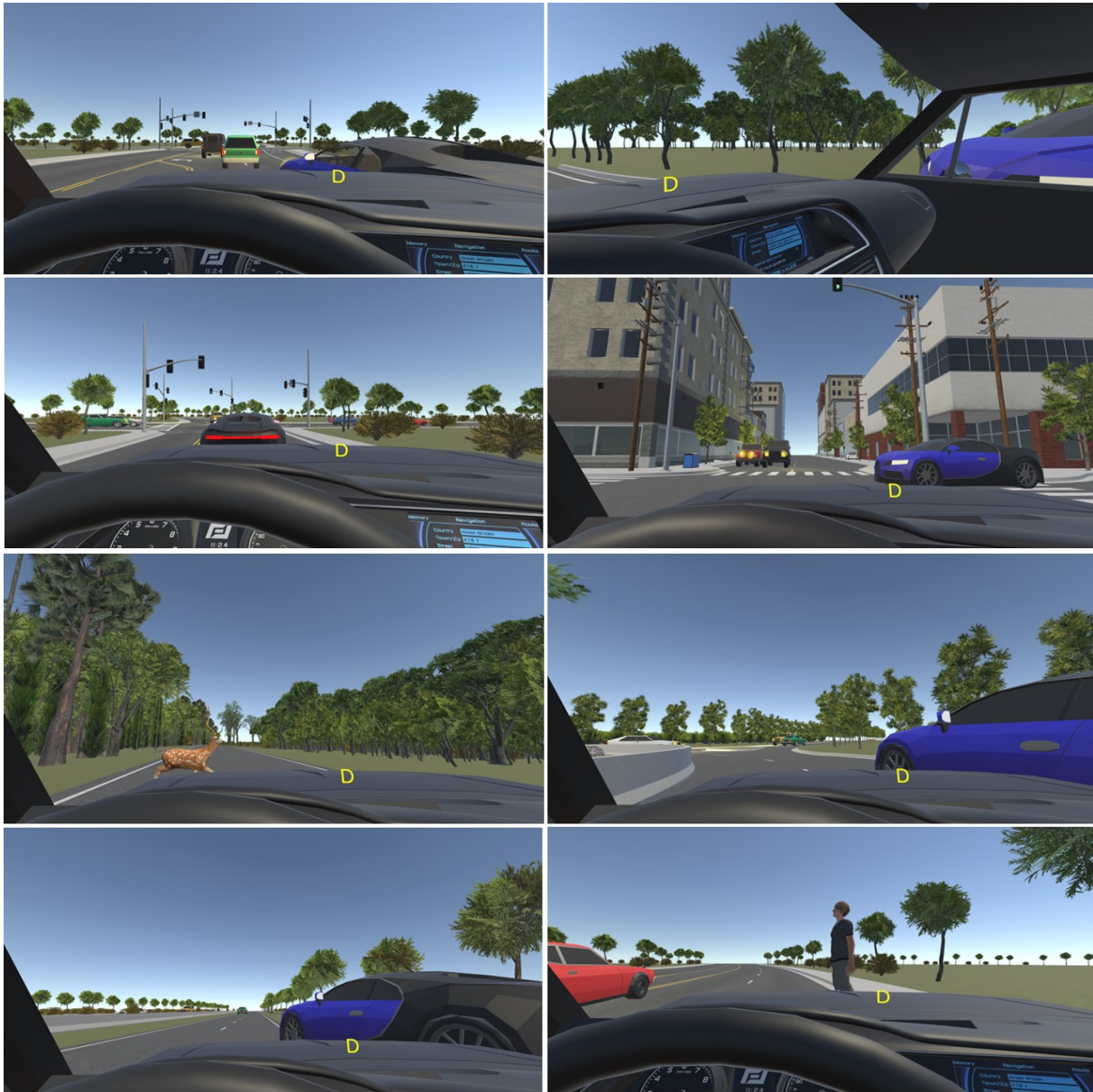
Fig. 3. NHTSA pre-crash scenarios implemented in our virtual reality driving simulation. Scenarios include Sudden Lane Change Interaction, T-Bone Crash, Sudden Vehicle Stop in Front, Vehicle Running Red Lights, Sudden Deer Crossing, Crash at Roundabout, Crash in Ramp Merger, and Jaywalking Pedestrian Crash (from left to right, top to bottom). These scenarios were designed to simulate various challenging driving situations mentioned in NHTSA pre-crash typology [10] to enhance the realism and effectiveness of the simulation. The letter D indicates driving modes (D/R)
