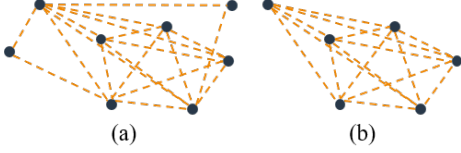
Fig. 7: Figure (a) shows all possible correspondence pairs. Figure (b) presents the obtained maximum consistency set.
