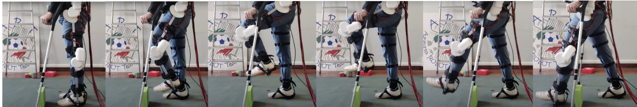
Fig. 7: Frame sequence related to one of the experimental trials (initial left step surpassing the big rectangle-shape object).
