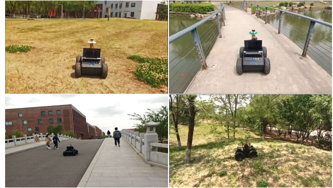
Fig. 1. The Bulldog, a four-wheel differential mobile platform, serves as the primary experimental vehicle to validate the robust exploration capabilities of PARE in various challenging terrains. Our experiments are strategically conducted across various environments, including steep slopes, flat bridges, dense forests, and arch bridges.
