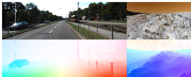
Fig. 2: Optical flow results of NeuFlow: on the left is a result from the standard KITTI dataset. On the right are results from a UAS flight overlow-contrast glacier images in the Arctic. Our approach is notable for both computational efficiency and speed as well as accuracy, as shown in Fig. 1.
