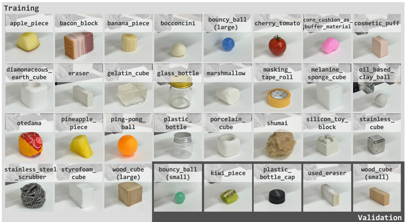
Fig. 4. Snapshots of the TactileReference dataset. It is used in two modules. In the tactile embedding network module, the dataset is split into 27 classes for training and 5 classes for validation. In the tactile-to-text database module, all classes of the dataset are used to construct the tactile-to-text database.
