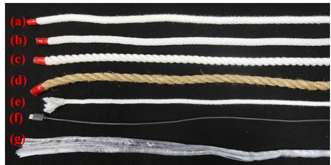
Fig. 10: Types of rope: (a)12-strand vinylon rope, (b)12-strand nylon rope(12mm), (c)3-strand vinylon rope(12mm), (d)3-strand hemp rope(12mm), (e)12-strand nylon rope (7mm), (f)cable, and (e)PP tape.
