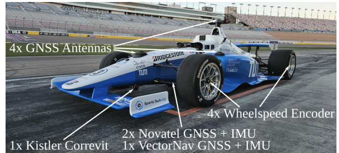
Fig. 1: Sensor Setup of the Dallara AV-21 race car used for data recording on the Las Vegas Motorspeedway.
