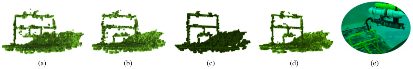
Fig. 2: a) Map generated with the Dead Reckoning b) Map generated with the SLAM and not corrected c) Map generated with Octomap d) Map generated with our method f) The pipe structure.
