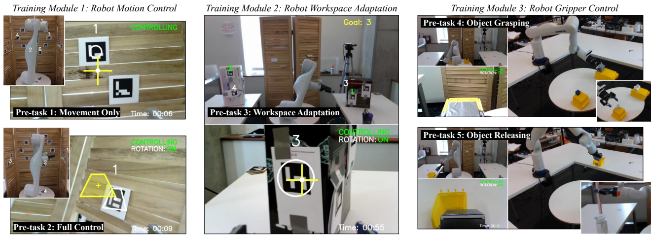
Fig. 3: We developed three interactive remote teleoperation training modules to assess and enhance telemanipulation capabilities. The robot motion control module, comprised of two pre-tasks, focuses on the aspects of movement and full control. The robot workspace adaptation module aims to improve arm ergonomics during remote teleoperation. The robot gripper control module includes two pre-tasks that focus on manipulating objects of various sizes and shapes and dropping them into a bin or precisely aligning them for insertion.
