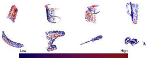
Fig. 5: Visualization of the shape features learned by the last layer of UOP-Net backbone on YCB objects.
