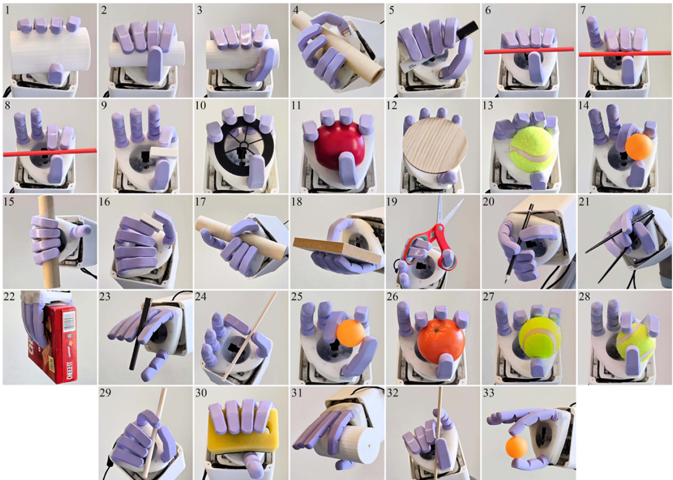
Fig. 9. Proposed soft hand is capable of realizing all 33 grasp postures of the GRASP taxonomy [59].
