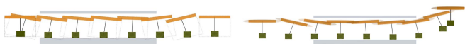
Fig. 7. Optimized trajectories by PolyFly for the ceiling-floor (left) and ceiling-wall (right) environments. The dashed lines are the polytopic approximation by PolySingle and the semi-transparent ellipse is the ellipsoidal approximation.
