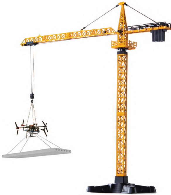
Fig. 1. Envisioned target application for stabilization of a crane-load system using a suspended underactuated multirotor platform.
