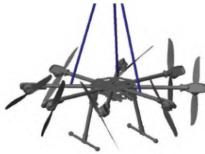
Fig. 8. Simulated omnidirectional multirotor platform suspended using cables.
