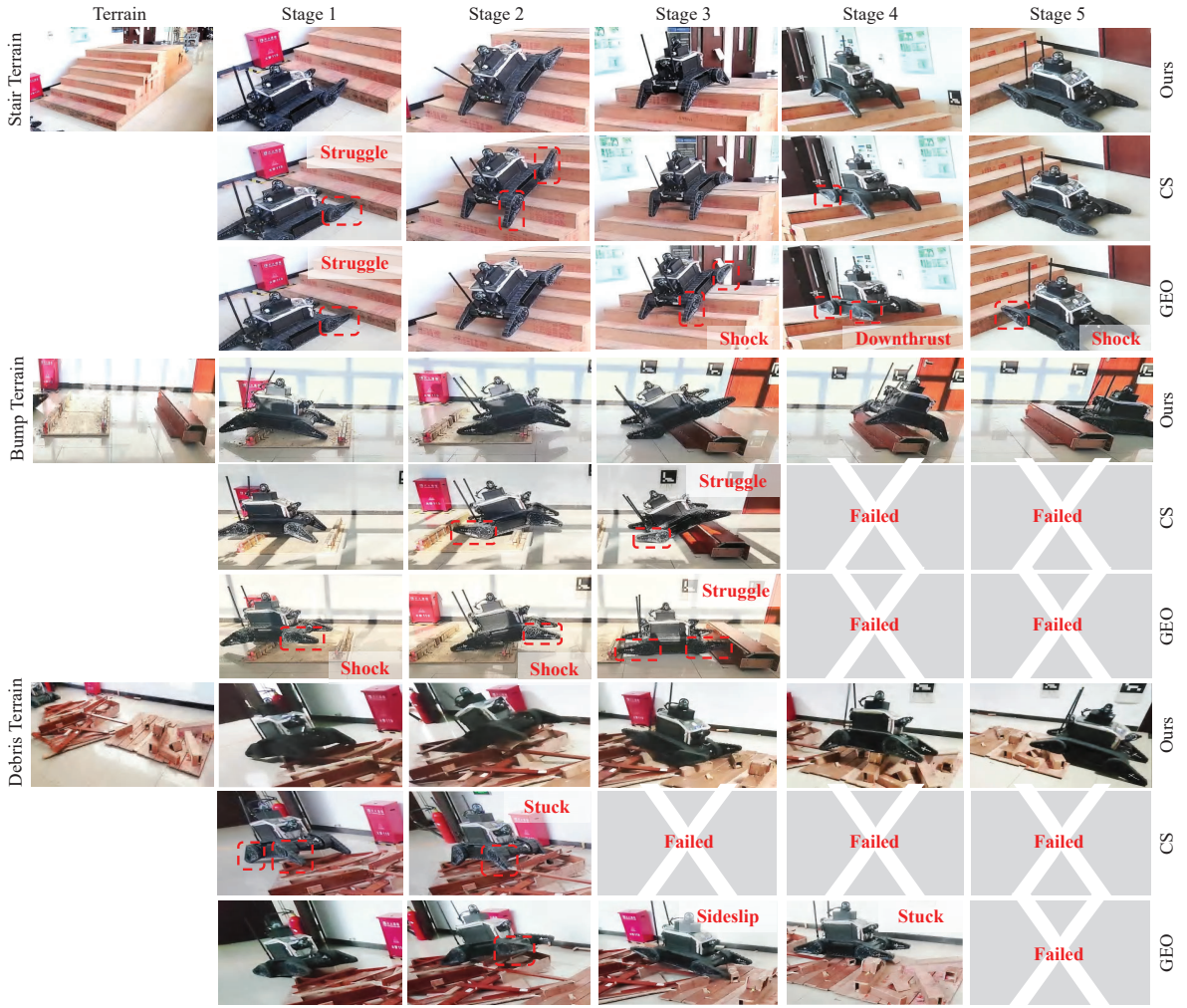
Fig. 23. Robot configurations when traversing three challenging terrains in real-world scenes. The red dashed boxes highlight improper flipper angles.
