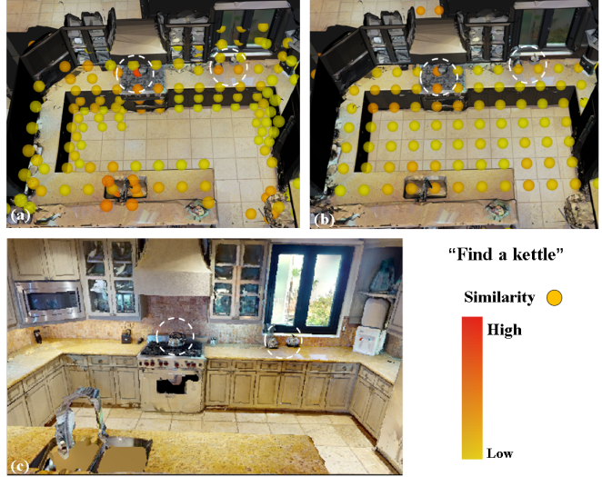
Fig. 4: Comparison of 3D and 2D feature map. (a),(b) is the result of 3D and 2D feature map, respectively; the colored spheres indicate the likelihood of target presence, where red denotes higher confidence regions. (c) is the scene, where targets are marked with a white circle in the figure.
