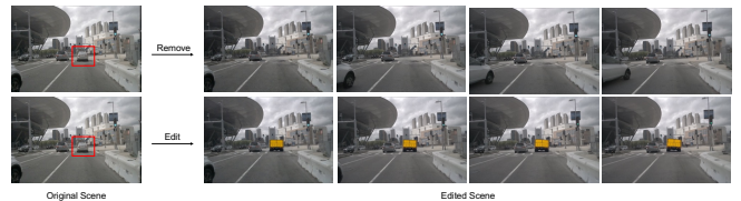
Fig. 7: Qualitative Results on Scene Editing. Our approach enables the removal or replacement of vehicles within a scene, allowing for the prediction of seamless future scenarios.
