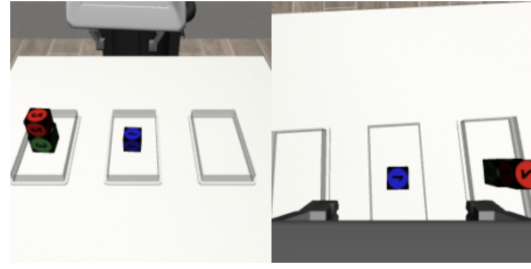
Fig. 2. Example observations from the dataset. Left: Agent-view RGB image. Right: Wrist-mounted camera RGB image.
