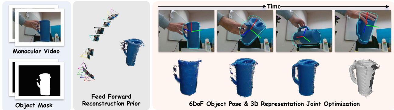
Fig. 1: Given a monocular RGB sequence and object mask, MGS-Track utilizes a feedforward network to obtain geometric priors, enabling 6-DoF pose tracking and 3D reconstruction of the target. Results are directly visualized by our method.
