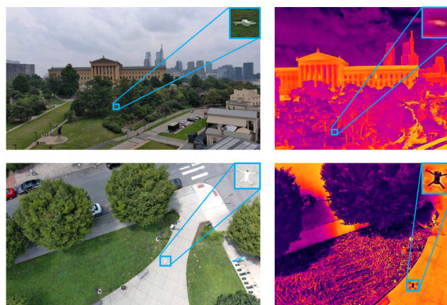
Fig. 4. Examples of thermal image pairs from the dataset. The RGB images are collected at 4K resolution, and the IR images are recorded at 640x512, centered relative to their RGB counterparts
