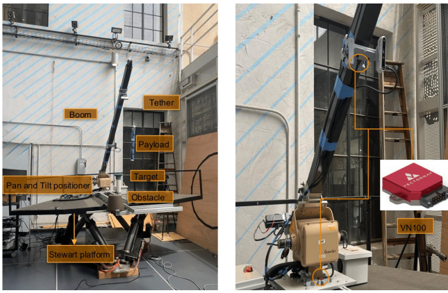
Fig. 3. Stewart-platform testbed. Left: Moving-base crane with target, obstacle, payload, and arm/tip cameras. Right: Base-mounted VectorNav VN-100 IMU supplying orientation and angular rates to the sliding window Hankel-DMD predictor.
