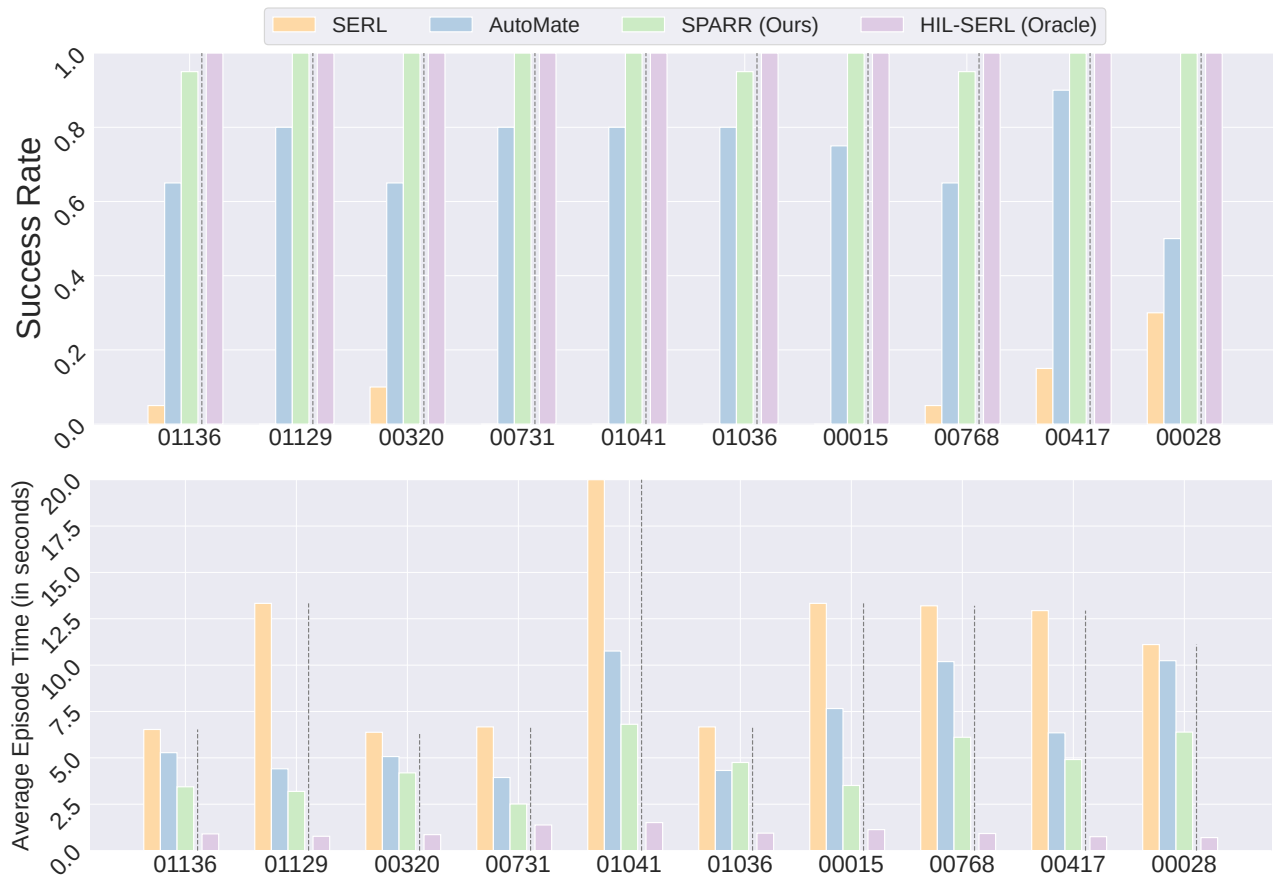
Fig. 4: Performance on 10 AutoMate tasks. We evaluate the success rate ( \uparrow higher is better) and cycle time ( \downarrow lower is better) averaged over 20 episodes. SERL, AutoMate, and SPARR (Ours) transfer simulation-trained policies to the real world without human effort, where SPARR achieves substantially higher success rates and shorter cycle times. HIL-SERL (Oracle) serves as an upper bound, assuming access to near-optimal human demonstrations and continuous human supervision.
