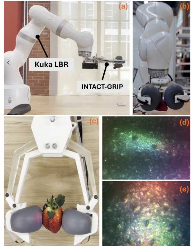
Fig. 1. (a) Integration of INTACT-GRIP with Kuka robotic manipulator while simultaneously obtaining texture images and safely grasping an asymmetrical strawberry; (b) Front and (c) top views of INTACT-GRIP safely gripping the strawberry with two inflated tactile sensing balloons; (d) left- and (e) right-side textural views of strawberry mapped by the inflated balloons of INTACT-GRIP.
