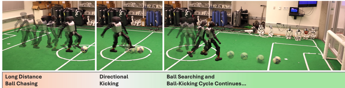
Fig. 1: The illustration of a complete ball-kicking cycle in the robust continual ball-kicking task.
