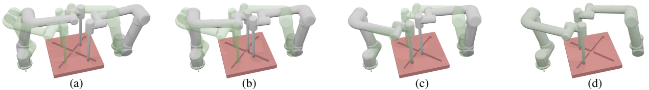
Fig. 6: An example of HaMMAR successfully solving a doorway-crossing task. The robots’ current configurations are shown in solid gray with their goals shown in transparent green. The sub-figures illustrate a single trial at different time steps, where the robots start from their initial configurations and get close to each other (a-b), wait until clearance (c), and then safely move towards their goals (d). The corresponding video demonstration is available in the supplementary materials.
