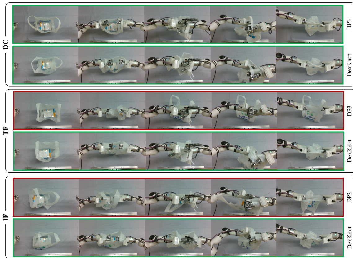
Fig. 5. Qualitative comparison of policy executions. Successes and failures are indicated by green and red bounding boxes, respectively. Top row: Both DP3 and DexKnot successfully complete the knotting task under Diagonal-Compressed (DC) deformation conditions. Middle row: In Twisted-Flat (TF) conditions, DP3 fails to thread the handle while DexKnot successfully accomplishes the task. Bottom row: In Inclined-Flat (IF) conditions, DP3 fails to thread the handle while DexKnot successfully accomplishes the task.
