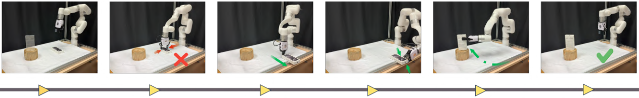
Fig. 4: Real-World Task Process Visualization. The goal is to place the box at the translucent target pose. Direct grasp fails because the box is slightly wider than the gripper. AdaptPNP replans by first pushing the box to the table edge and then grasping it from the side, successfully reaching the goal.
