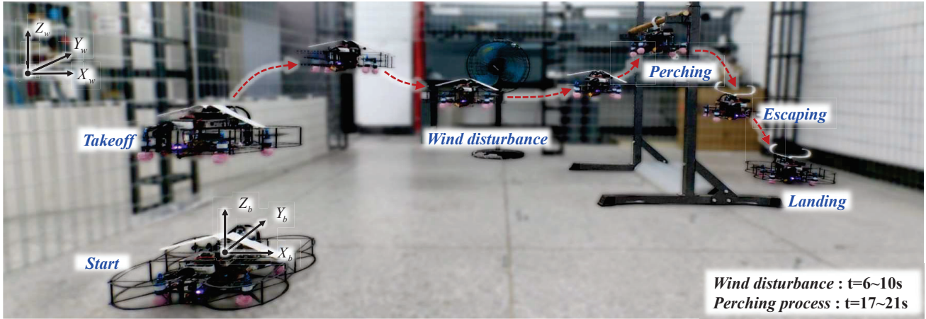
Fig. 6. Perching mission process. (Note: Illustration of the drone’s operational sequence includes takeoff, perching, escaping, and landing. During the process, an electric fan generates the wind disturbance to evaluate the effectiveness of the cascaded EHGO in maintaining stability.)
