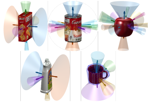
Fig. 10: Example of stable poses for YCB objects exhibiting various shapes. Arrows indicate the stable normals from StabPose, with their corresponding cones. For the non-convex mug, a slightly enlarged convex hull (blue) is shown.
