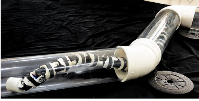
Fig. 1: Snake robot in the pipe.
