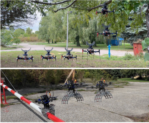
Fig. 10: SPARO’s modality and universality across different robots and mounting configurations. The same gripper enables successful perching on various platforms, confirming ease of integration and repeatability.
