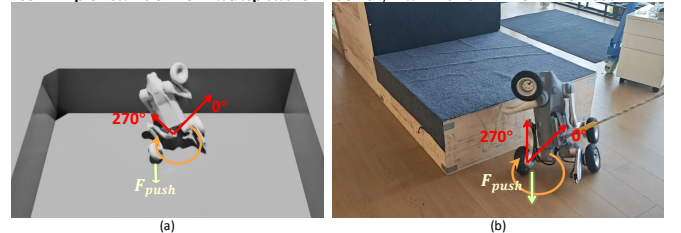
Fig. 6: High platform climbing without DC-Motor constraints. The rear thigh joint is at joint limit and will generate large torque to jump highly. (a) In simulation (b) In real world.
