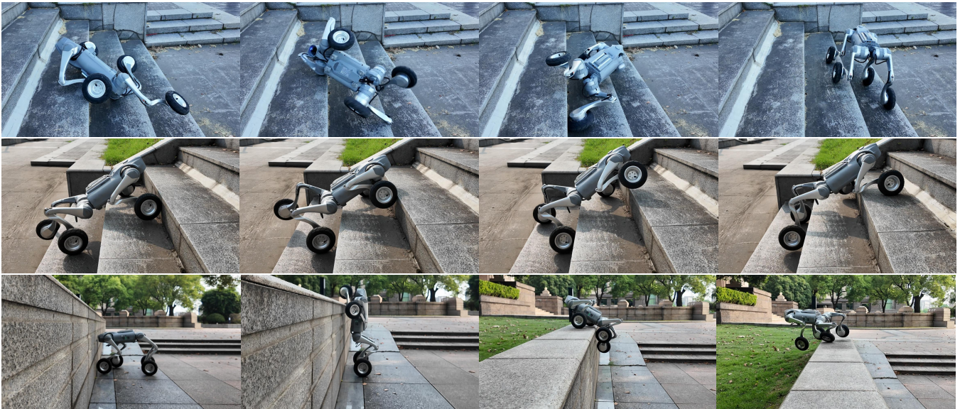
Fig. 7: Real-world evaluations of individual skills. Top row: Fall recovery on stairs. Middle row: Ascending 20-cm-high stairs. Bottom row: Climbing an 80-cm-high platform.
