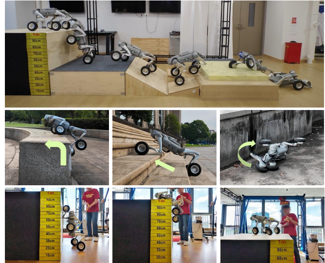
Fig. 1: Real-world demonstrations of MUJICA on the wheeled-legged robot. Top row : automatic skill switching during continuous locomotion. Middle row : execution of three representative skills, including high platform climbing, stair ascent, and fall recovery. Bottom row : snapshots of the robot climbing onto a 1-m-high platform. The results highlight MUJICA’s ability to perform diverse skills and seamlessly transition between them without external perception.
