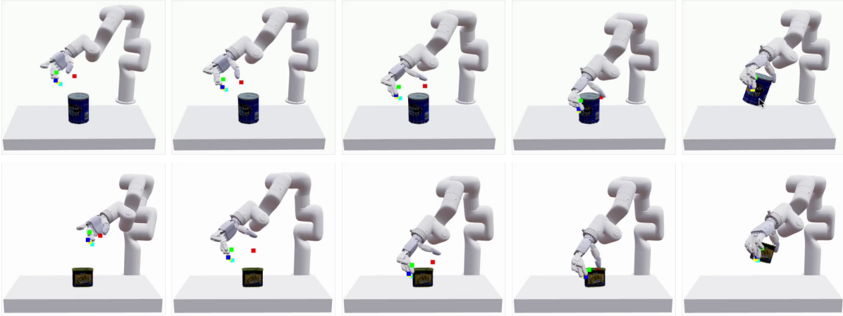
Fig. 3: Qualitative Results. A policy trained with our approach successfully picking up two objects. The colored points show the next predictions of \Pi_h . Such predictions are temporally smooth and guide the policy towards fast grasping and lifting (better seen in the videos available at our supplementary webpage https://dynamicsprediction.space ).
