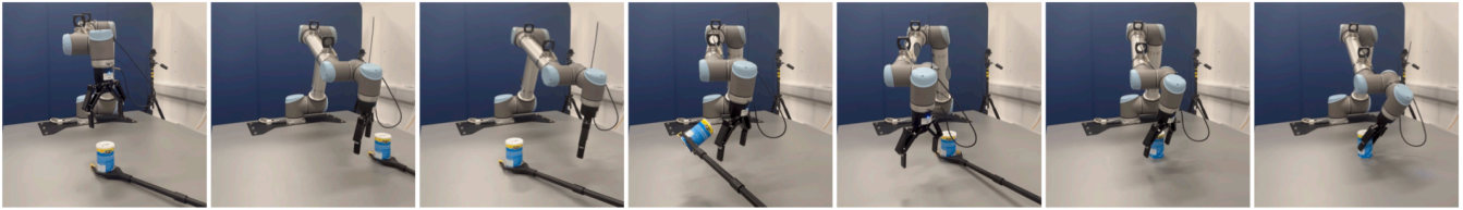
Fig. 10: Grasp-MPC execution for moving objects. Grasp-MPC adapts in real time to track and grasp moving target objects, capabilities that open-loop approaches lack.
