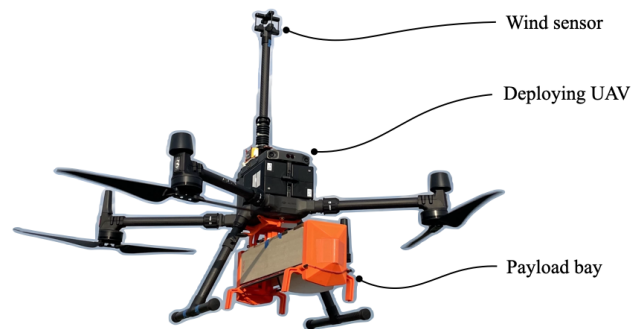
Fig. 7. Deployment UAV used in trials, equipped with wind sensor and payload bay.
