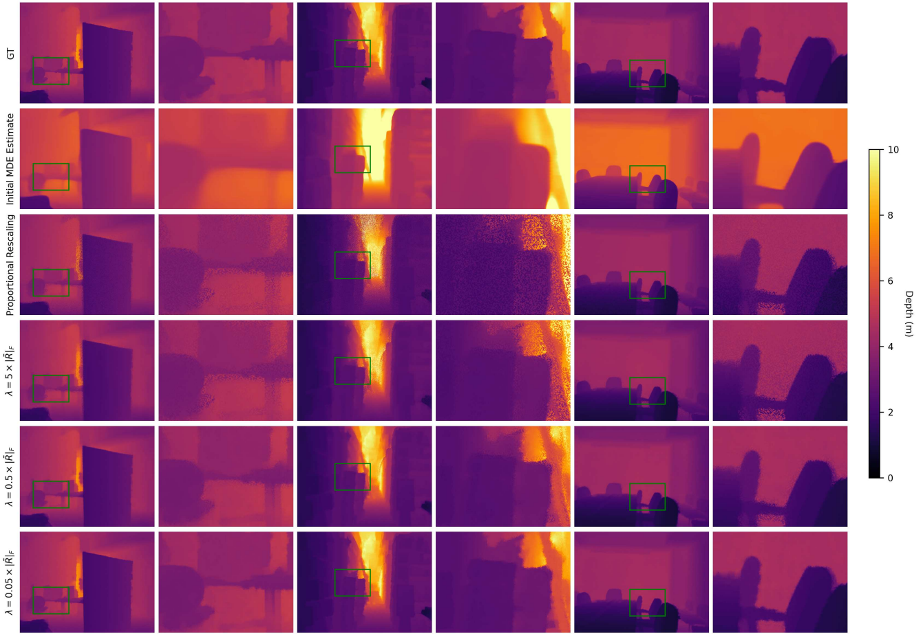
Fig. 4: Depth maps from selected NYUv2 scenes, comparing ground truth, initial MDE estimate and the rescaled depth using our compressed sensing pipeline at different values of \lambda
